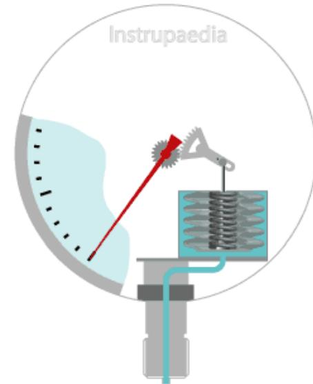
Fig. shows the hydraulic method of transmission, which is commonly used.
